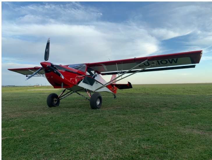
KFA Safari – Rotax 915iS with FP-Propeller
